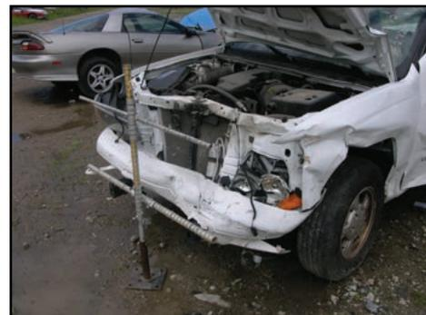
A stuck accelerator caused the crash that damaged this vehicle.
